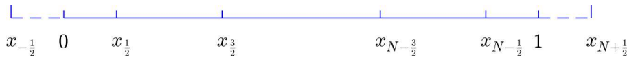
Figure 1: The 1-D spatial grids, where x_{-\frac{1}{2}} and x_{N+\frac{1}{2}} are two ghost points.
